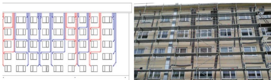
Fig. 16.6 Ventilation ducts in façade insulation layers: schematic view with red supply air ducts and blue exhaust air ducts (left), and photo (right)
