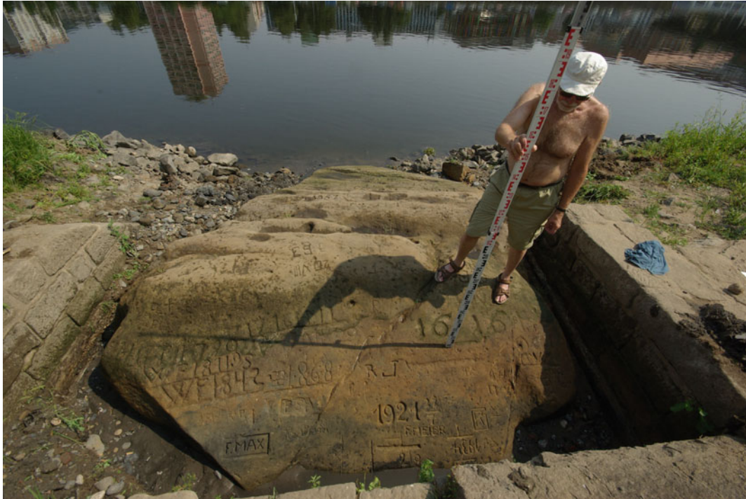
Fig. 10.17 Hunger stone with low water marks of the River Elbe at Decin/Czech Republic. Photograph Elleder
