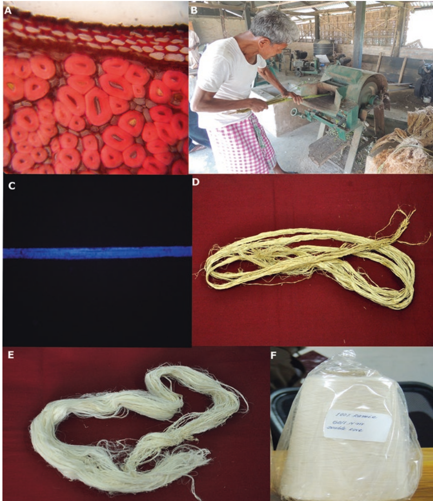
Fig. 5.4 Ramie fiber: structure and properties. (a) Cross-sectional view of ramie fiber cells in phloem, (b) Decortication of ramie fiber, (c) Single fiber strand (ultimate fiber), magnification 100x, (d) Decorticated fiber, (e) Degummed fiber, (f) Ramie yarn
