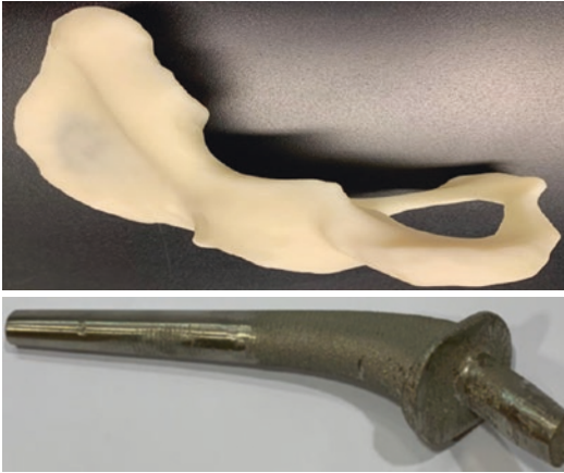
Fig. 11.6 A 3-D printed model for a pelvis and a neck femur implant
