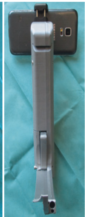
Fig. 11.13 Novel videoscope (Shalliscope) second prototype printed by 3D printer as proof of concept
