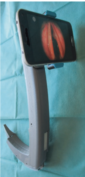
Fig. 11.13 Novel videoscope (Shalliscope) second prototype printed by 3D printer as proof of concept
