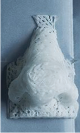
Fig. 6.8 3D printed nose for surgical planning, intraoperative guidance, and surgical simulation
