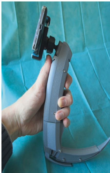
Fig. 11.13 Novel videoscope (Shalliscope) second prototype printed by 3D printer as proof of concept
