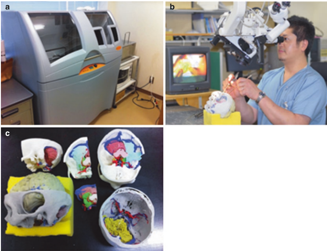
Fig. 6.6 The 3D color printer (Zprinter Z Corporation, Inc.); (a) the color-printed plaster models based on CG data modified through IVS (b). Realistic surgical sensa-
