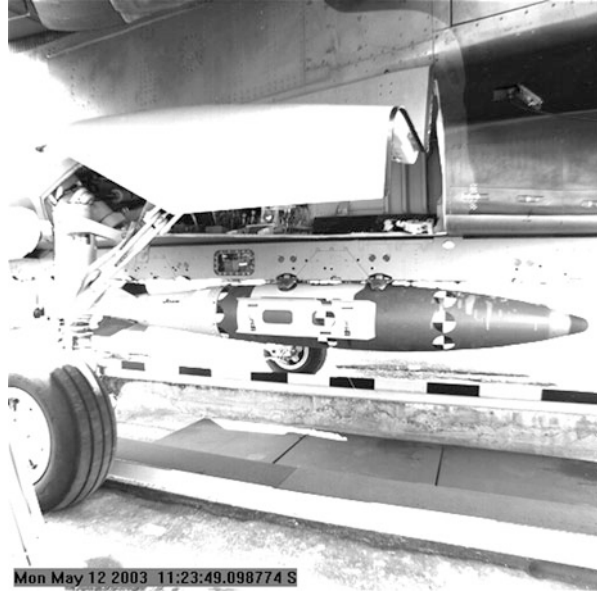
Fig. 10 Pit drop trials during Joint Direct Attack Munitions (JDAM) integration on Tornado
