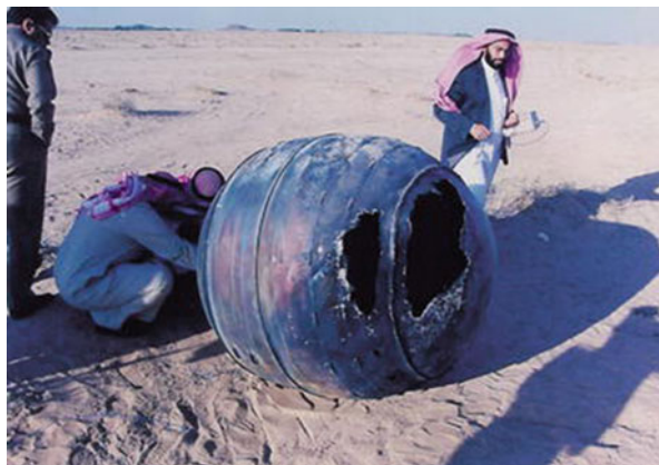
Fig. 5 Reentered titanium motor casting of third-stage Delta 2 (Saudi Arabia, 2001) (NASA courtesy)
