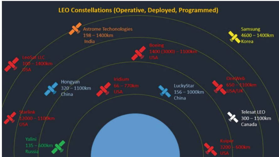
Fig. 2 Operative, on deployment, and planned constellation on LEO region
