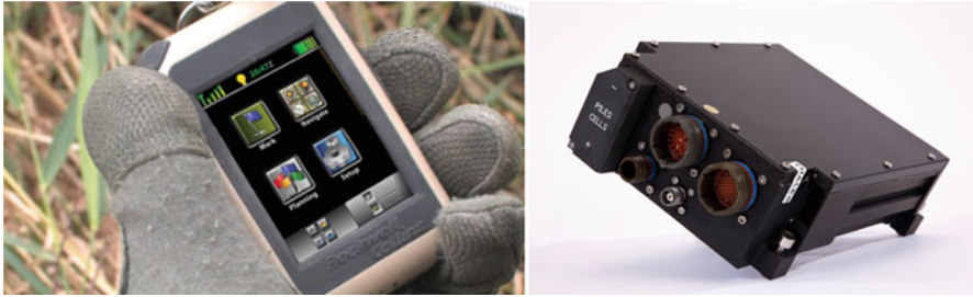
Fig. 3 Left: Hand-held micro Defense Advanced GPS Receiver (DAGR). (© Collins Aerospace). Right: TOPSTAR M for avionics platforms. (Photo Thales © E. Raz)
