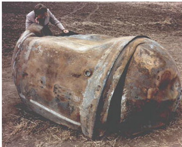
Fig. 4 Stainless steel propellant tank of second-stage Delta 2 reentered launch vehicle (US, 1977) (NASA courtesy)
