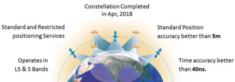
Fig. 3 Constellation and features of NavIC
