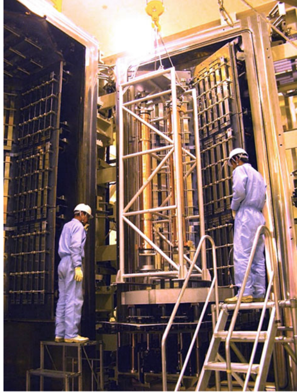
Fig. 38 Brazing two accelerator columns in a vacuum furnace
