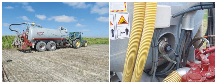
Fig. 2 A slurry tanker equipped with disc injectors ( left ) and detail of the nitrogen rate control system based on electrical conductivity ( right ). (Photos by C. Cantero-Martínez)
