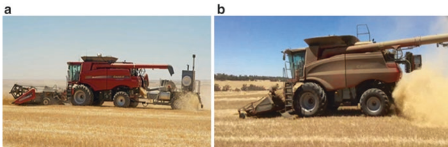
Fig. 3 (a) HSD and (b) iHSD systems developed for chaff processing and weed seed destruction during harvest
