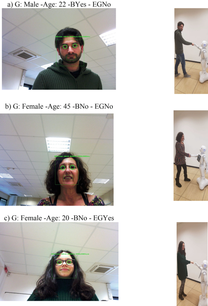
Fig. 4. Three examples of interaction with the Pepper robot. The robot recognizes soft biometrics traits of the interacting subject and greets with a customized behavior.
