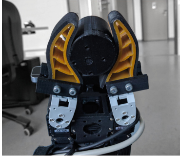
Fig. 1. Flexible fingers without sensors while grasping an object. The fingers’ deformation is clearly visible. Each finger consists of two flexible bands that meet at the top to form a triangular shape and four horizontal ribs .
