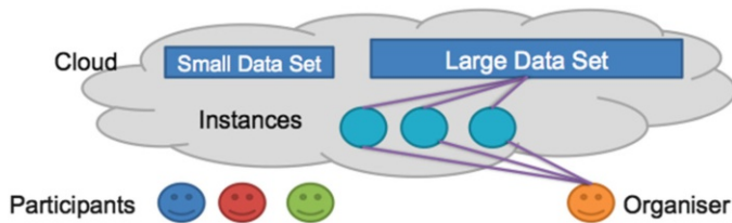
Fig. 3 On the competition deadline, the organiser takes over the instances containing the software written by the participants, links them to the large data set, performs the calculations and evaluates the results (image taken from Hanbury et al. 2012)
