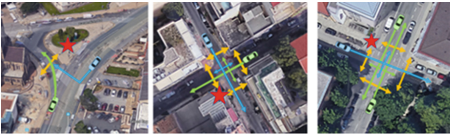
Fig. 1. An aerial view of the intersections used at Leeds (left), Athens (middle) and Munich (right). Yellow arrows represent the location and direction of pedestrians’ crossings. The blue and green lines represent the direction of travel for vehicles. The red stars represent the location of a group of two observers who used the mobile app to record observed behaviour (for further details see [2]).
