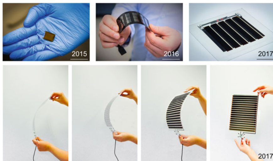
Fig. 10.15 The evolution of demonstrators by Saule technologies: (2015) An ink-jet printed perovskite solar cell. (2016) A perovskite solar module made of single cells externally connected in series. (2017, top) Ink-jet printed flexible perovskite solar module (2017, bottom) An A4 paper-sized, ink-jet printed perovskite solar module, capable of charging portable electronic devices. Courtesy of Saule Technologies
