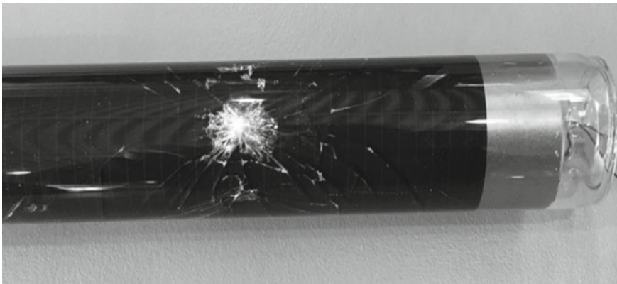
Fig. 11.10 The solid encapsulation helps to optically match the CIGS cells to the glass tubes, and also to hold the shards if some break
