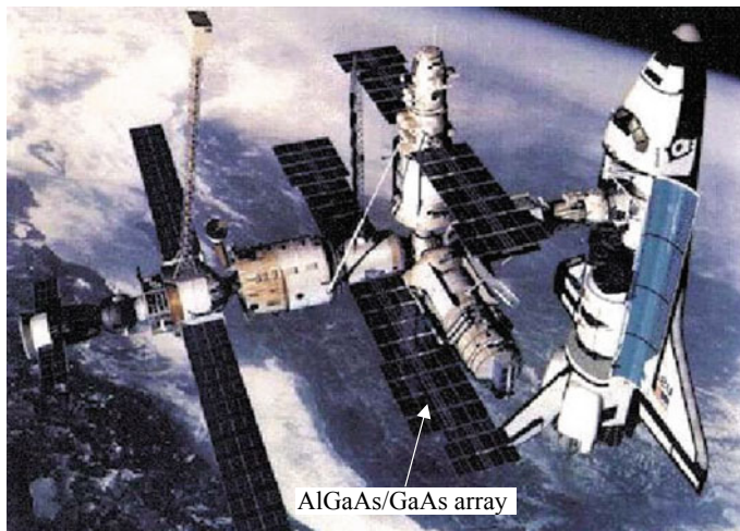
Fig. 8.1 Command module of “MIR” space station was launched into orbit on March 13, 1986 with PV array based on AlGaAs/GaAs SCs developed at Ioffe Institute and fabricated in NPO “Kvant”. The array has been operating during the 15-year space station span-time
