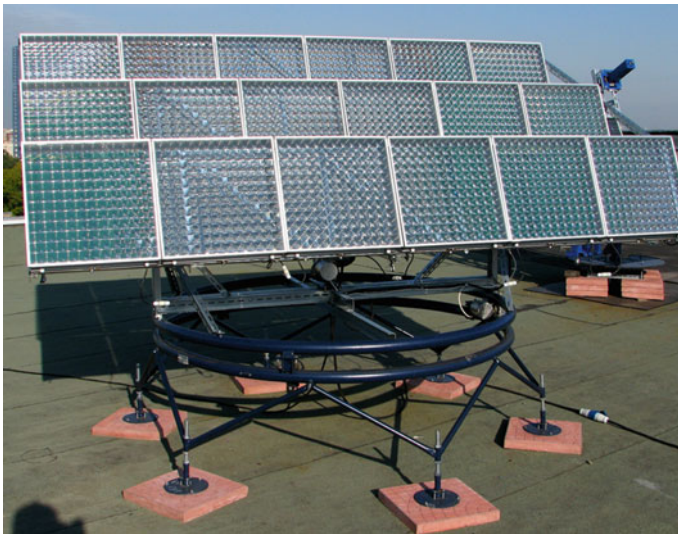
Fig. 8.12 PV tracker equipped with Fresnel lens concentrator modules
