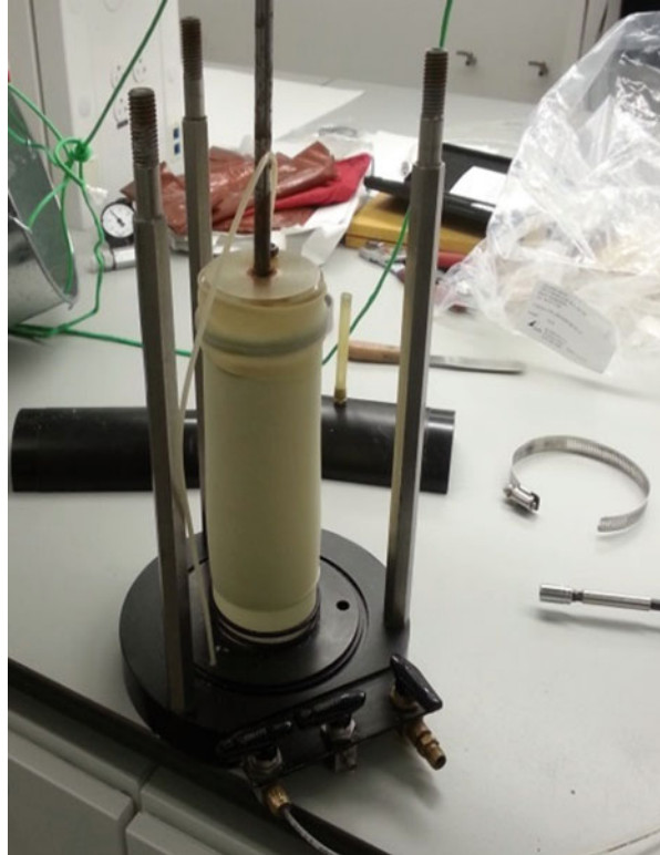
Fig. 3.7 Prepared sample subject to vacuum
