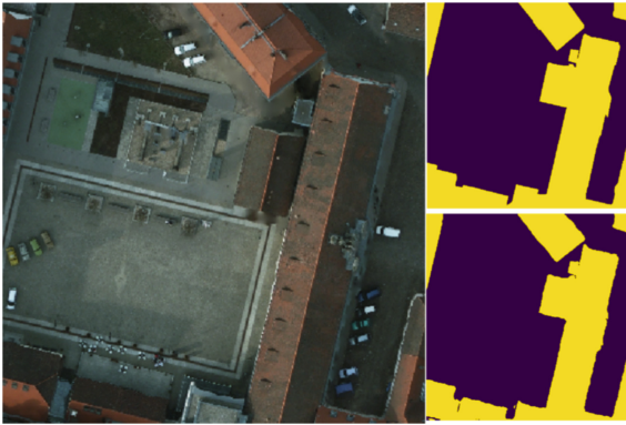
Fig. 10. Example of segmentation (loss— L_{BF_1, IoU} ). Left: original orthophoto, top right: ground truth segmentation, bottom right: predicted segmentation
