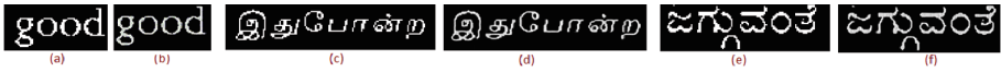
Fig. 3. (a), (c), (e): English, Tamil and Kannada input images originally scanned at 200 dpi. (b), (d), (f): the corresponding output images created by our CTCS architecture with increased perceptual quality.
