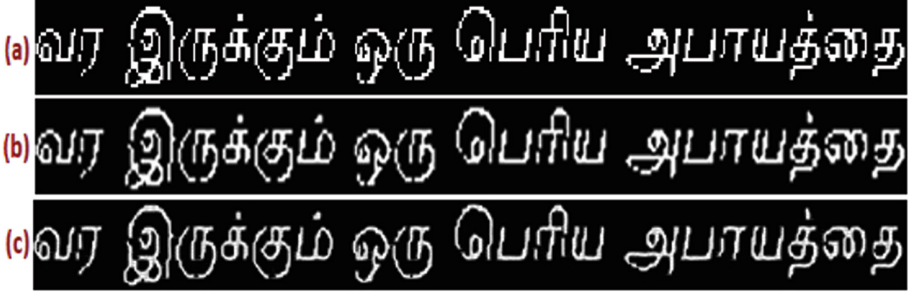
Fig. 4. (a), (b): Input binary image and the corresponding output images (gray scale) created by our CTCS architecture. (c): image in (b) after gamma correction [20], displaying significantly improved perceptual quality and enhanced readability.
