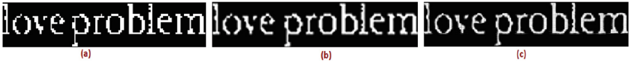
Fig. 7. (a), (b), (c): Input English, bicubic interpolated and the corresponding output images created by our CTCS architecture with increase in perceived quality and ease of readability. In the word ‘love’ character ‘o’ and in the word ‘problem’ character ‘m’ is broken in both input and the bicubic interpolated output. But the same is reconstructed in the CTCS architecture
