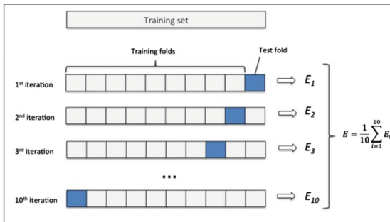
Fig. 8. Schematic diagram of cross validation
