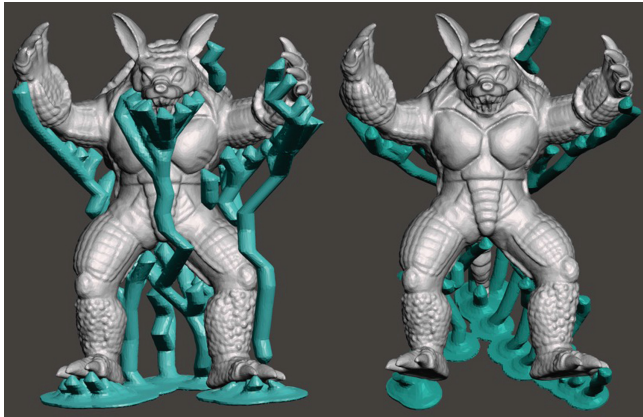
Fig. 5. “Optimal” and “default” printing directions for “Armadillo”.
