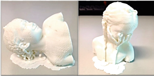
Fig. 2. 3D printed model from different support structure placement.
