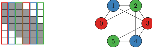
Fig. 1. Sparsity pattern of the Hessian (left) and the corresponding adjacency graph (right) with colors obtained by acyclic coloring for the function from (6) (Color figure online)
