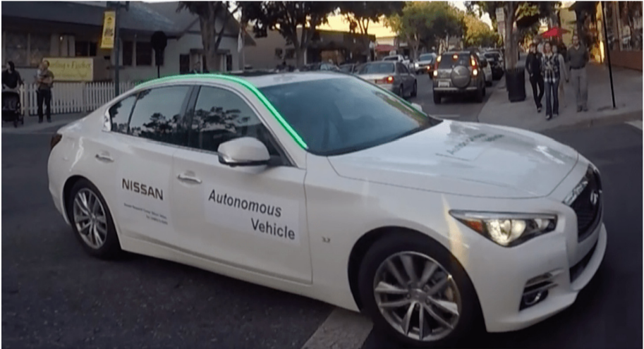
Fig. 3. Intention Indicator prototype used in public road test
