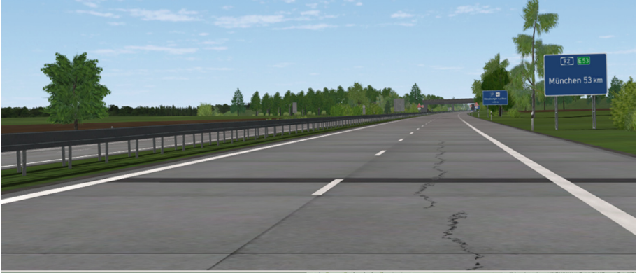
Fig. 3. Virtual highway with road damages
