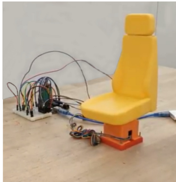
Fig. 3. Low-fidelity scaled prototype for user testing
