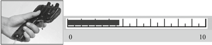
Fig. 3. Handset control (left) and visual feedback (right) for the online-measurement of perceived safety while driving highly automated. Higher values indicate higher perceived safety.
