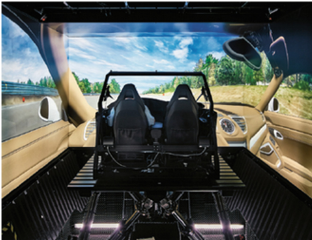
Fig. 2. Driving simulator of Porsche AG with motion dynamics
