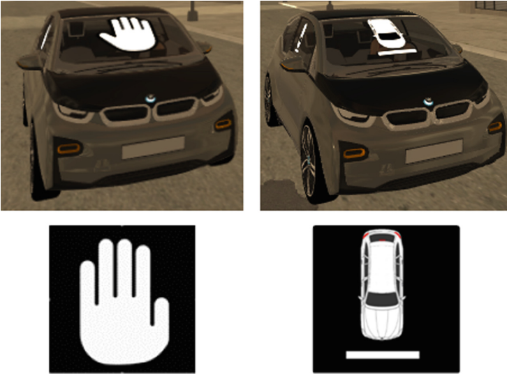
Fig. 3. Icons for intentions (left: “Pass” with open hands, right: “Give Way” with stopping car)
