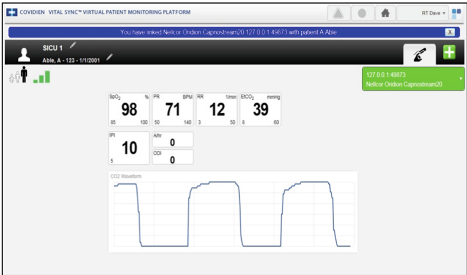
Fig. 1. Screenshot of the patient view of the Vital Sync™ Virtual Patient Monitoring Platform 2.4; all four vital parameters (SpO 2 = peripheral capillary oxygen saturation, PR = pulse rate, RR = respiratory rate, EtCO 2 = end-tidal carbon dioxide) and the IPI (= Integrated Pulmonary Index) score are displayed [19]
