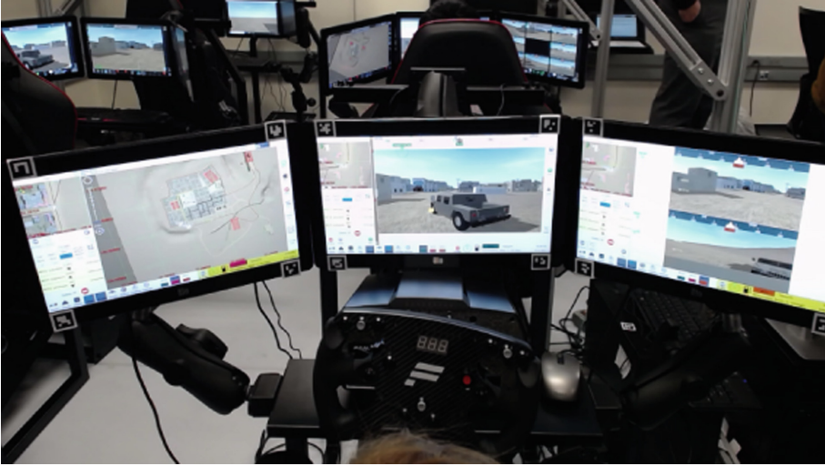
Fig. 1. A picture of the MEL-SIL setup. Each crew station is equipped with a driving simulation with 3 touch-screen monitors. Each monitor screen provides different interfacing displays. The left screen contains high-level map information for coordination and route planning; the middle screen provides a live view of the manned or unmanned vehicle driving environment and status; the right screen shows a 360° view from sensors mounted on the vehicle. The interfaces are modular, allowing crew members to configure them dynamically to suit the current task requirements.
