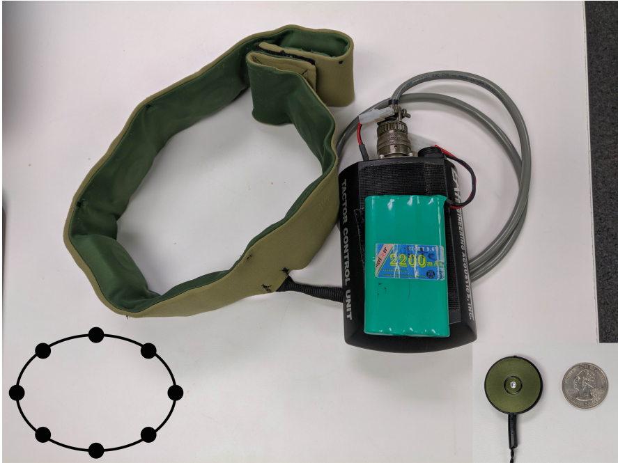
Fig. 2. A picture of the tactile belt and C2 factor used in the study. A schematic depicting location of the tactors on the belt is also included.
