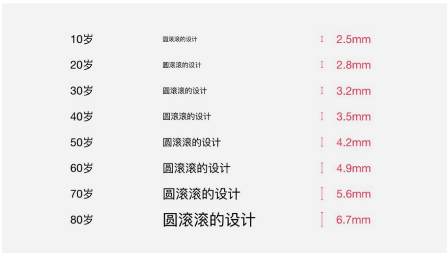
Fig. 2. Schematic diagram of smallest identifiable sizes of characters for different age groups
