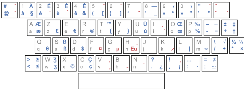
Fig. 1. The new French keyboard standard (NF Z71-300). Special characters (blue) and diacritic marks (red) were added to the old AZERTY layout. More information about the new standard can be found on https://norme-azerty.fr (Color figure online)
