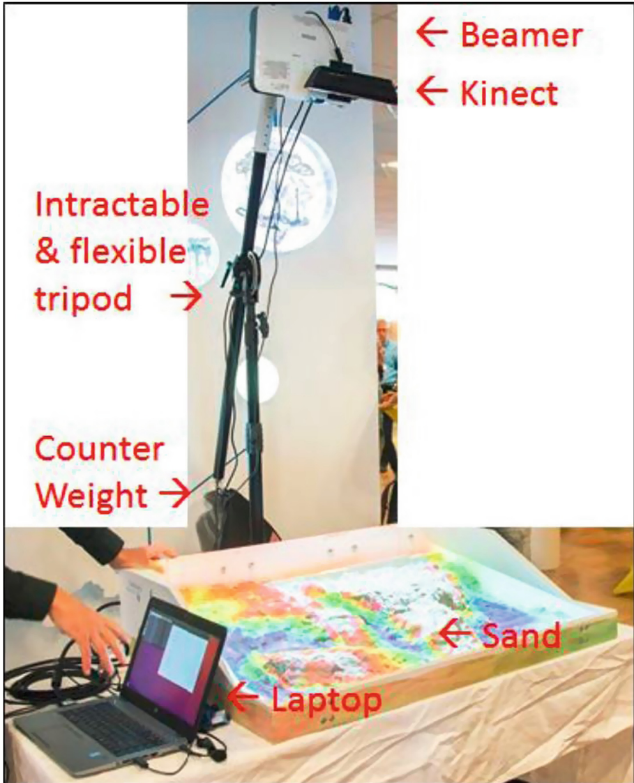
Fig. 2. SandBox setup and interface (photo from [74]). The SandBox uses a Kinect to measure the geometry of the sand, representing a river stretch. Molding the sand into a new shape changes the schematization used by the hydrodynamic model and a beamer projects the model's output back on the box of sand.
