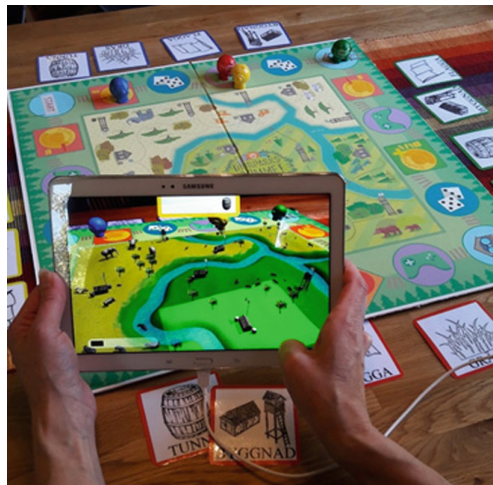
Fig. 2. The final prototype, with the tablet in AR-mode, showing an animated 3D-view of the two dimensional game board. (©Niklas Torstensson)
