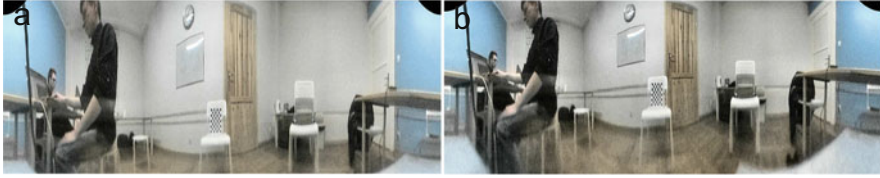
Fig. 2.5 Rectified panoramic images: constructed using only the inverse projection (a), and constructed using our improved method (b)
