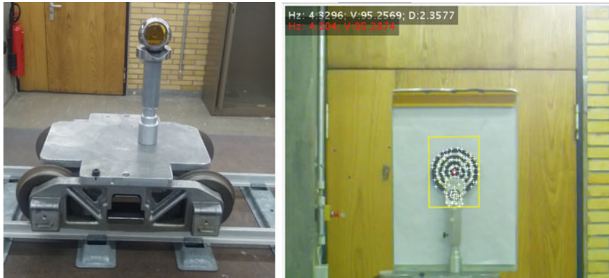
Fig. 5.31 Moving trolley with laser tracker reflector (SMR) (left) and the target with feature points as identified by the IATS (right)
