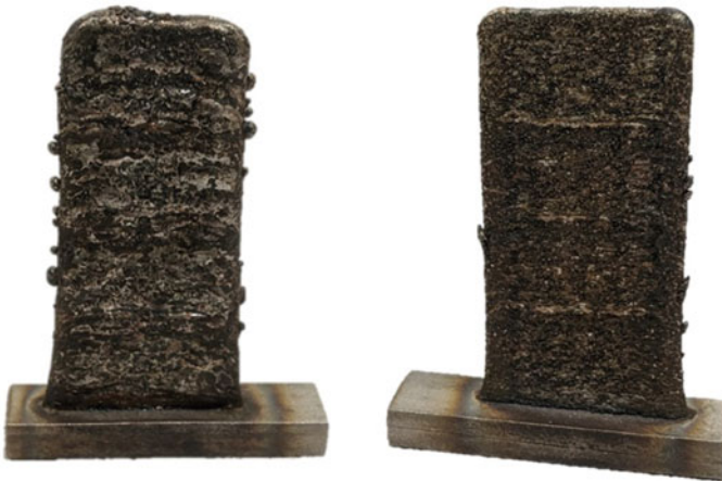
Fig. 22.2 Thin wall deposits fabricated without (left) and with (right) the control of feedback systems
