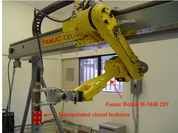
Fig. 11.3 Industrial robot used to validate the proposed approach
