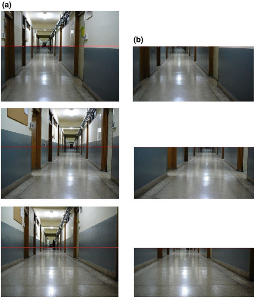
Fig. 20.3 Testing image sets for finding the MDGP with different camera height values, from up to down the height value were 1 m, 0.75 m, and 0.50 m above the ground plane. (a) Input images, the red line indicated where the MDGP was localized. (b) Output image after removing the information above the horizon line
