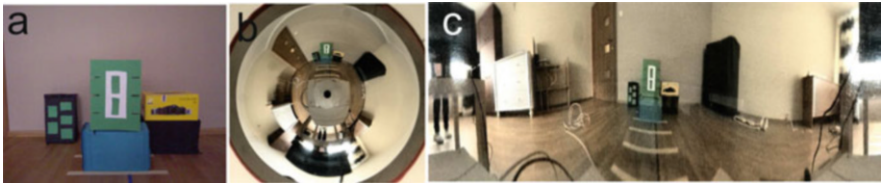
Fig. 2.13 Different images for one of the scenes: perspective camera image (a), omnidirectional camera image (b), and panoramic image (c)
