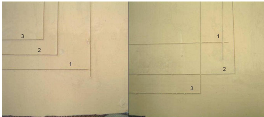
Fig. 11.16 Comparison of closed paths traced by simple geodesic mapping (1), interpolated geodesic mapping (2), and virtual projection (3)
