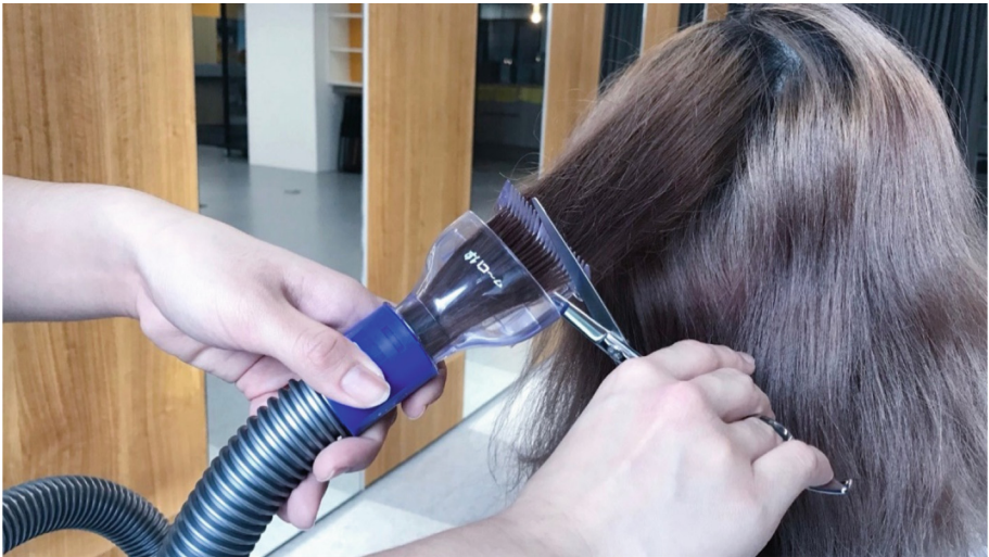
Fig. 8. "Sui-comb" vacuumed hair comb
