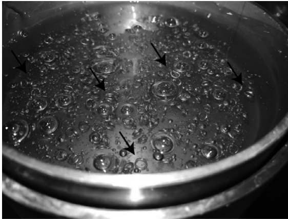
Fig. 3. Sedimentation of circular fibres (marked with arrows) with a diameter of 4.1 mm and a material diameter of 0.5 mm. Bubbles are present due to manual mixing of the material.
