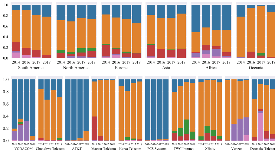
Fig. 4. NAT type distribution by continent in 4 different years (top) and NAT type distribution by the top 10 providers in 4 different years (bottom). Colors represent types as defined in Fig. 3. (Color figure online)
