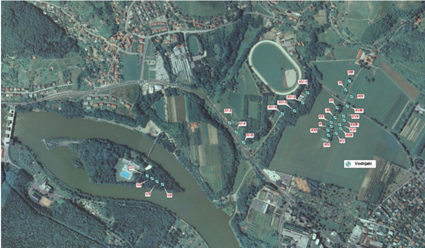
Fig. 4.6 Existing wells of the I. phase of active protection (Kopač 2008)
