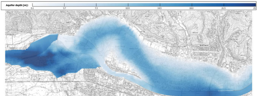
Fig. 4.9 Contour table of the model layer thickness (Kopač and Vremec 2017a, b)
