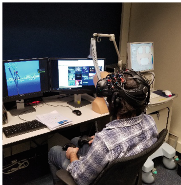
Fig. 6. fNIRS and HMD setup for the experiment
