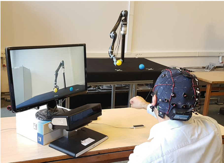
Fig. 4. Object manipulation based on Leap Motion controller and Jaco robotic arm
