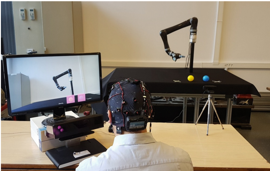
Fig. 3. SSVEP-based object selection
