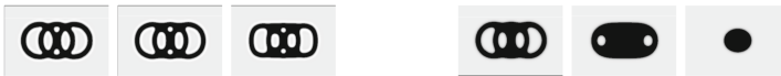
Fig. 2. Alteration after the same iteration numbers of the phase fields when w = 10 , left: the balanced phase field - interfaces are barely moved; right: the Ginzburg-Landau phase field: interfaces are displaced significantly. Weights are set according to (21) and (2) for the balanced model and the Ginzburg-Landau model respectively.
