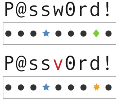
Fig. 1. Transparent Mask example inspired by Gruschka and Iacono’s paper [8]. The colorful symbols (blue star, green diamond) represent a hash of the previous characters in a password. A typo in the preceding characters would result in a different symbol appearing, as shown when the “w” is mistyped as a “v”. (Color figure online)
