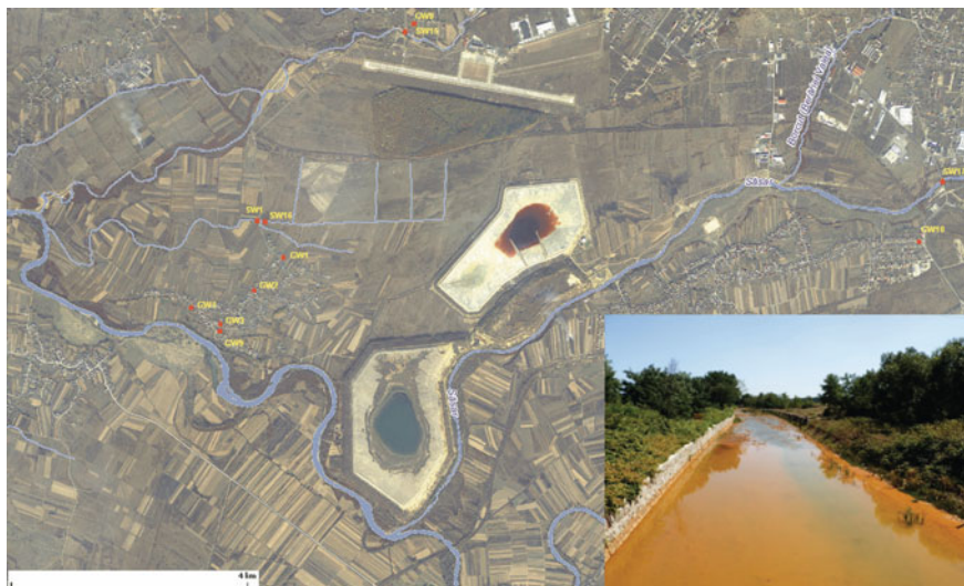
Fig. 3.33 Pollution of the Sasar River, in Baia Mare area and leaks of \text{Fe}(\text{OH})_3 from Aurul and Bozânta tailing ponds (2012) [115]
