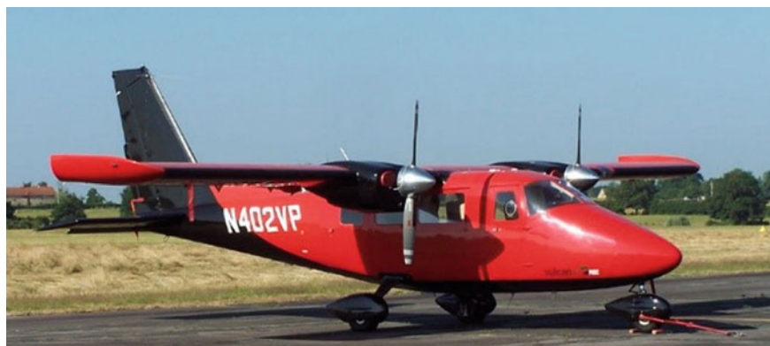
Fig. 8.3 Parten Avia plane for LiDAR (DEM- LIDAR: PARTENAVIA P3; Owner: APEI sa; Engine: 2×; LYCOMING 180 CV; Max Altitude: 25 000 Ft; Speed: 145 kts; Equipment: complete IFR/BR nav; LiDAR scanning hatch; Autonomy: 5 h)
