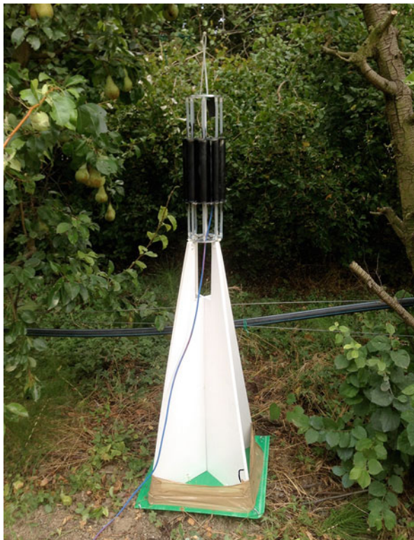
Fig. 19.5 A prototype bimodal trap with a pheromone dispenser, female vibrational signal (FS2) playback and a device administering electric shocks for killing the attracted bugs. Photo: Aya Ibrahim
