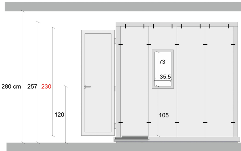
Fig. 3. Modular small room system as full-scope simulator
