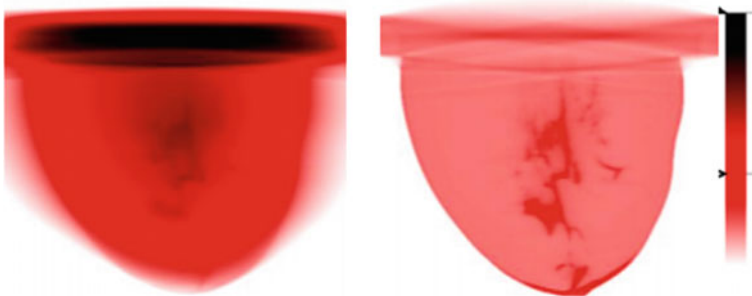
Fig. 41.1 Reconstruction of a simulated breast phantom, assuming monochromatic 35 keV X-ray beam, using the FDK analytical algorithm (left) and the iterative MLEM algorithm with 15 iterations (right)
