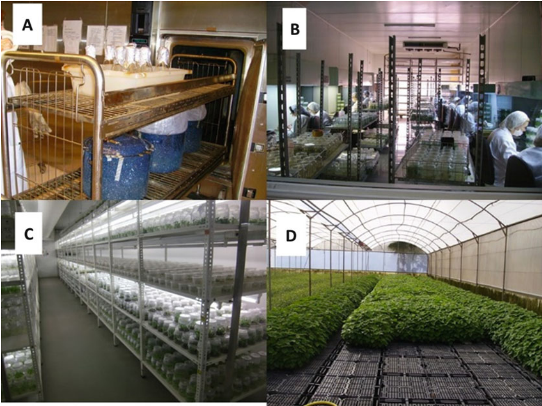
Fig. 3.4 (a) Industrial autoclave, (b) operators working at the culture room, (c) climate chamber with micropropagated plants in flasks, (d) greenhouse with acclimated plants
