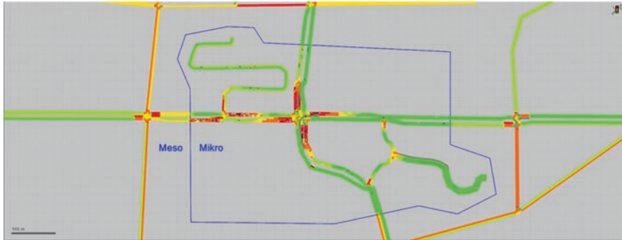
Fig. 7.1 Example of hybrid (meso + micro) simulation of traffic in PTV Vissim (source: [11])
