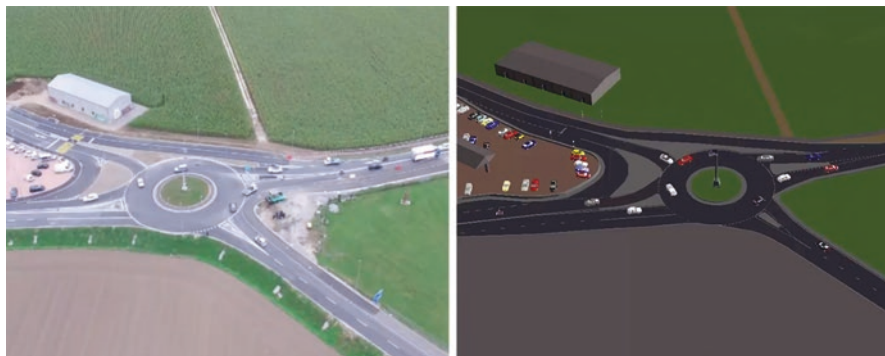
Fig. 7.8 Example of utilisation of DataFromSky for a calibration simulation model for more precise capacity estimation (source: [41])
