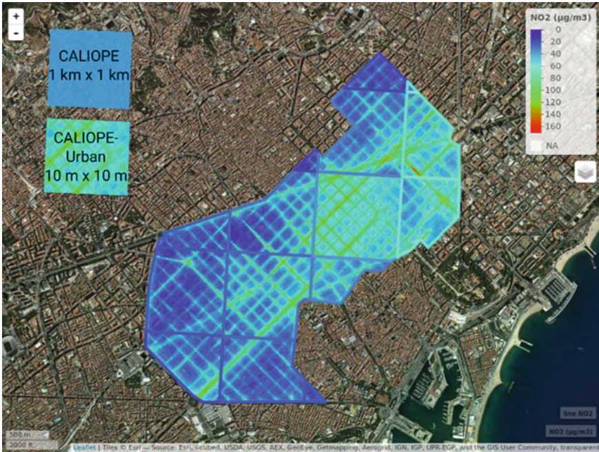
Fig. 27.1 NO 2 hourly level at 8 am (UTC) on 9th April 2013. Squares represent mesoscale 1-km grid cell values and the inside content street-scale concentrations
