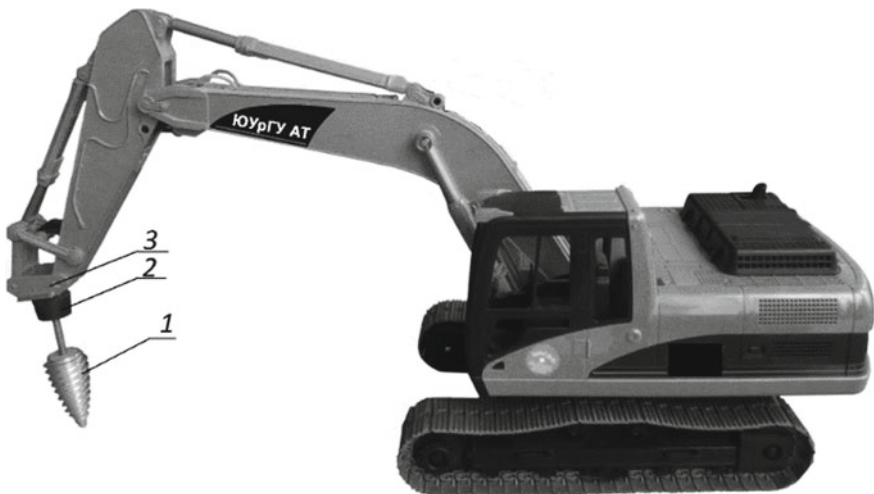
Fig. 6 Conical roller on the basis of a hydraulic crawler excavator. 1—Working body, 2—hydraulic motor, 3—traverse
