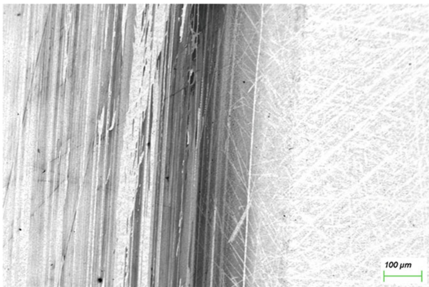
Fig. 2 SEM image of the friction track formed in DOS with 3% LCOA medium
