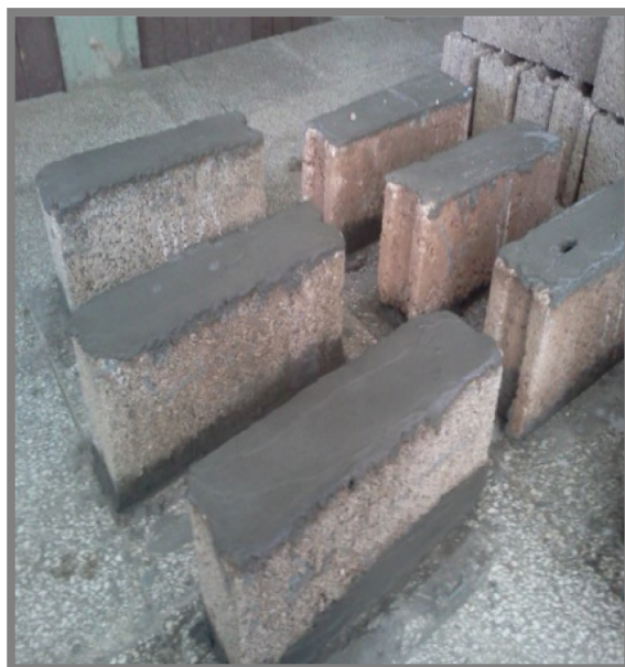
Fig. 1 Blocks made with LC 3 ready to be tested in compression
