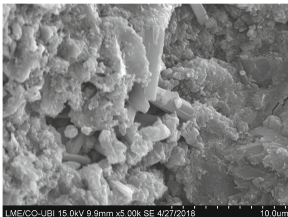
Fig. 4 SEM image of a Portland cement carbonated binder fracture
