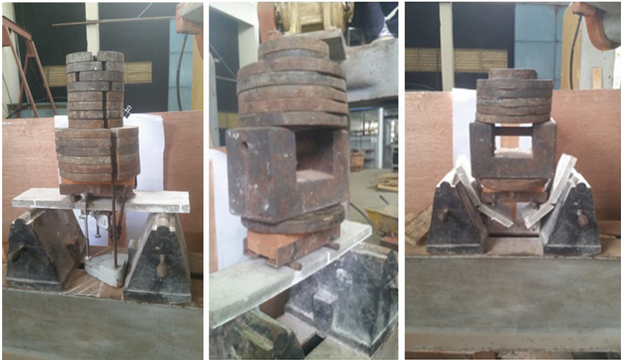
Fig. 4 Placement of loads (weights) and breakage of the specimen due to failure of the mortar
