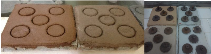
Fig. 3 Samples elaborated for the adhesion test
