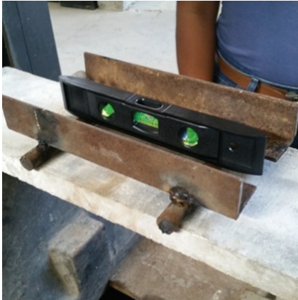
Fig. 6 Attachment to distribute the load in two points
