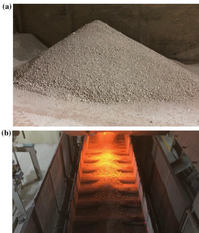
Fig. 2 a The selected kaolinitic clay dried, 90 ton. b The kaolinitic clay thermally activated
