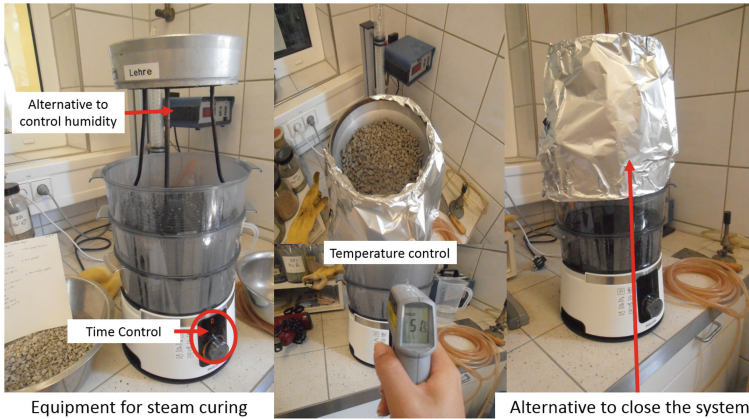
Fig. 2 Steam curing system
