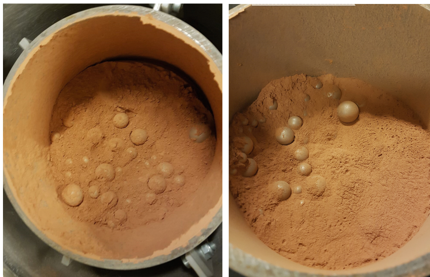
Fig. 1 Photographs of ground clay after 60 min incorporating (from left to right) no grinding aid and 0.15% PCE-based grinding aid
