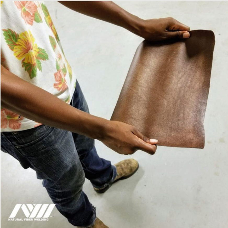
Fig. 2.5 Mirum™ is 100% plant-based leather-like composite. NFW is able to produce scalable materials that do not use harmful plastics like polyvinyl chloride and polyurethane. NFW believes ‘vegan’ should mean ‘plants’ not ‘petroleum’ nor ‘plastic’. (own source)
