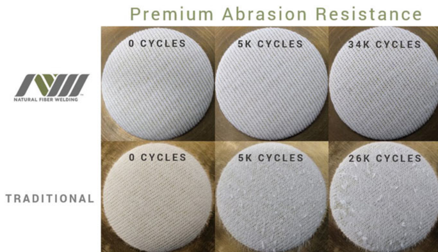
Fig. 2.3 Martindale abrasion testing results for Clarus™ jersey knits produced using Welded Cotton™ composite yarns and from conventional upland cotton control fabrics. Clarus™ fabrics continue to look and feel great long after traditional fabric controls have developed both pills and holes. (own source)
