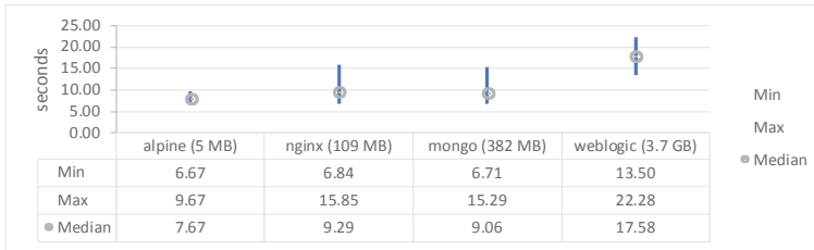
Fig. 2. Container recreation time for a container failure.
