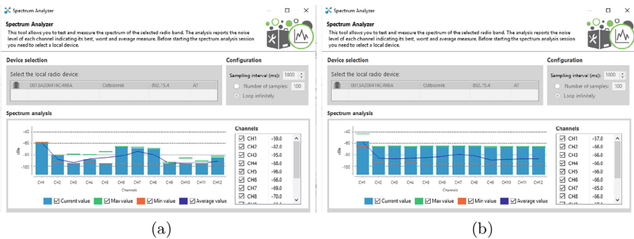
Fig. 6. The XCTU XBee spectrum analyser results: (a) without jamming, (b) with jamming
