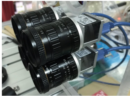
Fig. 2. Camera-array used for taking images for motion-tracking by DIC method
