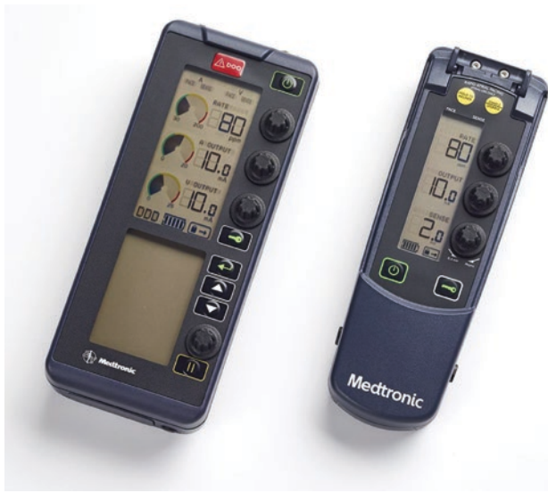
Fig. 52.1 Temporary dual-chamber and single-chamber pacemakers. (Reproduced with permission of Medtronic, Inc.)
