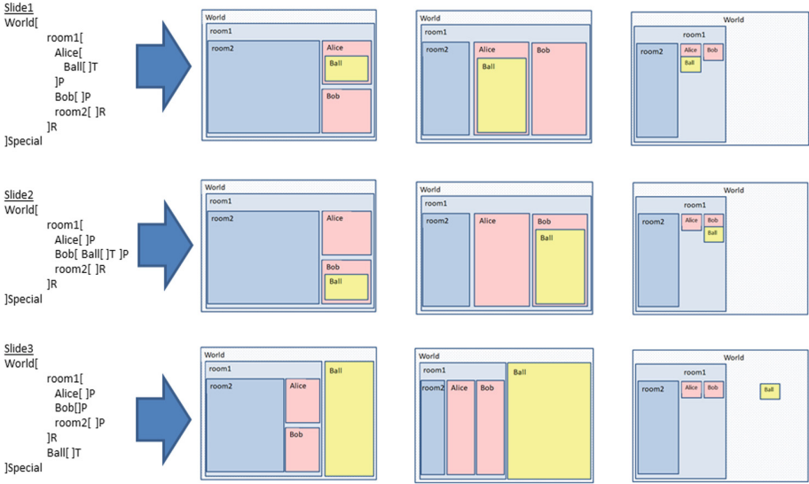
Fig. 4. The first column from the left is the textual representation of Fable slides; the second column is the rendering according to nested sticky nodes version 1, and the next two columns are rendered according to version 2 and the export to PPT layout algorithm.
