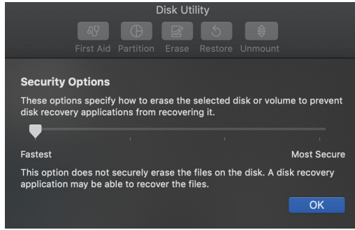
Fig. 3. macOS 10.14 dialogue to select Security Options when erasing the USB stick with Disk Utility . The lower description changes as different options are selected on the horizontal slider.
