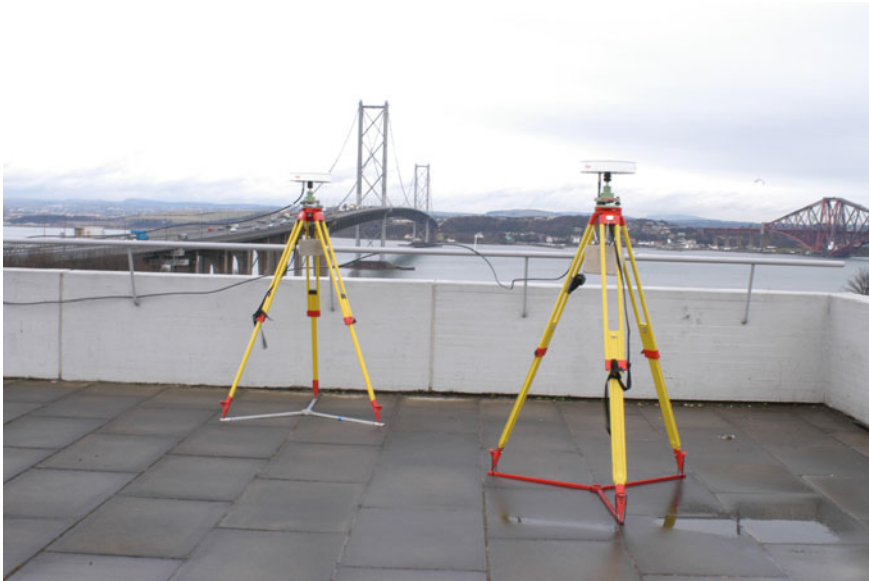
Fig. 12.39 Forth Road Bridge in the UK, with two Leica SR530 dual frequency GPS receivers utilising AT503 lightweight choke ring antennas acting as the reference stations. (Note the queuing traffic on the southbound carriageway)
