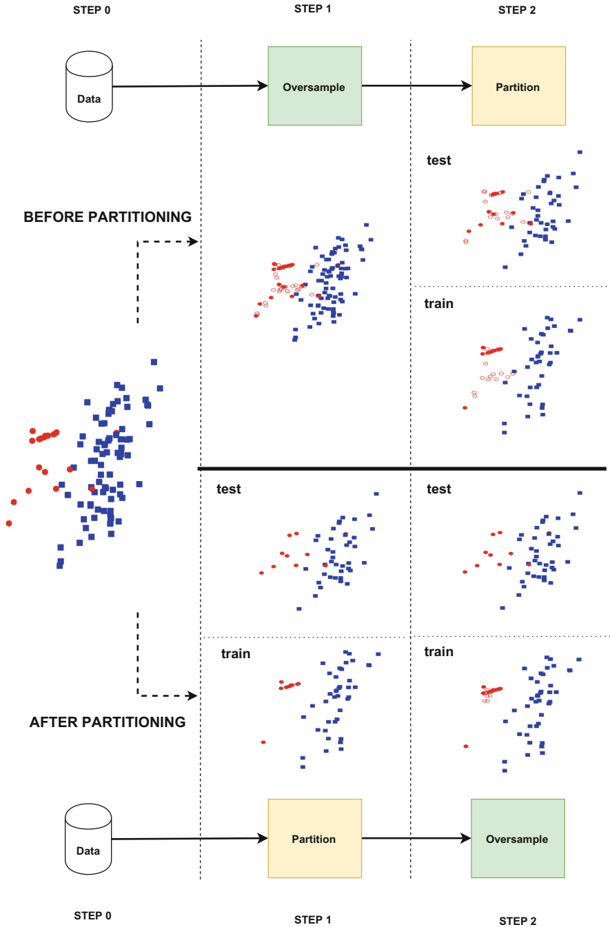
Fig. 1. Comparing the impact of applying over-sampling prior to data partitioning to applying over-sampling after data partitioning on a two-dimensional classification problem.
