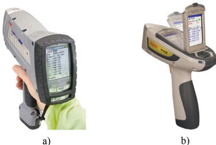
Fig. 4 Some examples of portable XRF analysers, (a) Oxford X-MET5000 Handheld XRF Analyzer (Oxford 2019) and (b) Thermo scientific XRF analyser (Thermo 2019)
