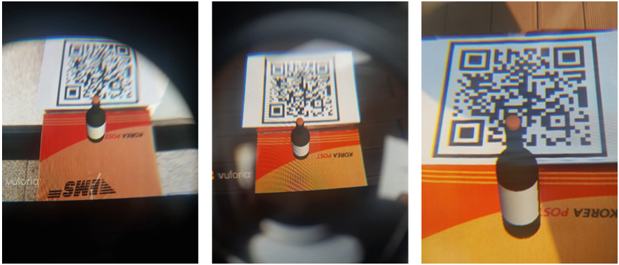
Fig. 4. Looking at an augmented object (bottle) with ClosedAR, Indoor (left), Outdoor low (middle), and Outdoor high (right) – p
