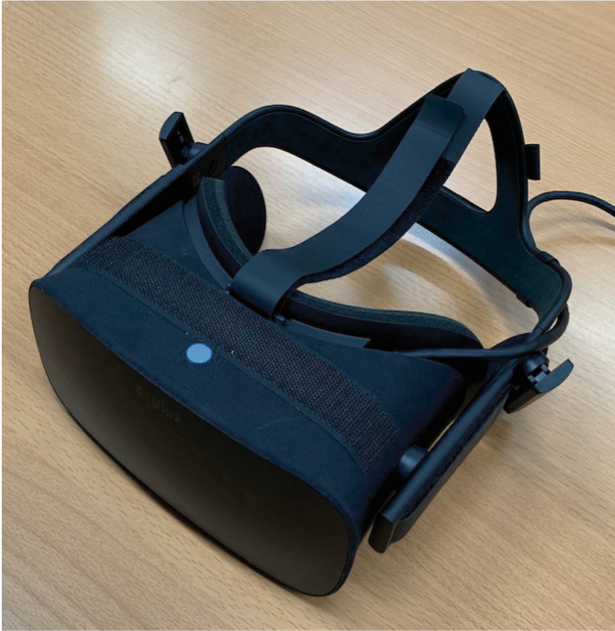
Fig. 3. Oculus Rift CV1 with hook-and-loop fastener
