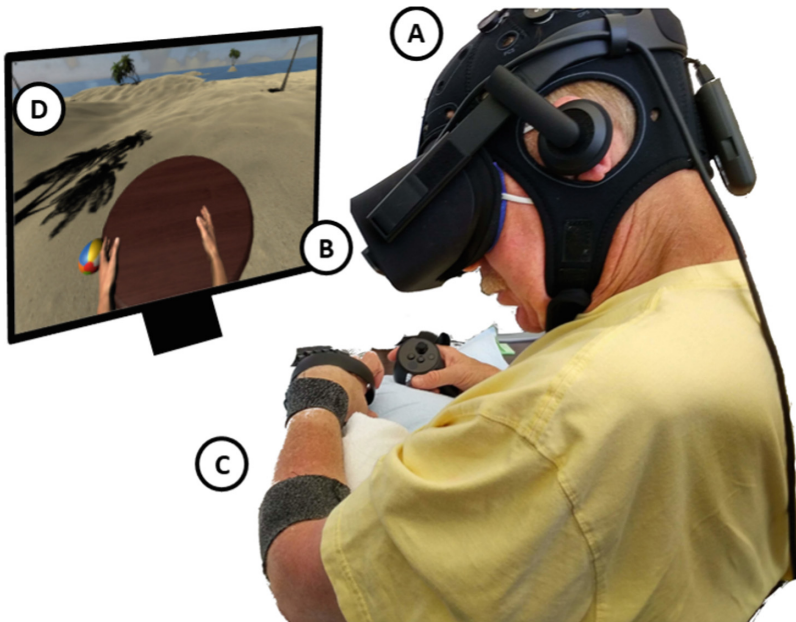
Fig. 1. System architecture: (a) EEG system with 8 electrodes over the motor and somatosensory areas, (b) Oculus Rift HMD delivering the VR feedback, (c) 4 EMG sensors over target muscles of the affected arm, (d) the dedicated desktop computer running the VR task and data acquisition.
