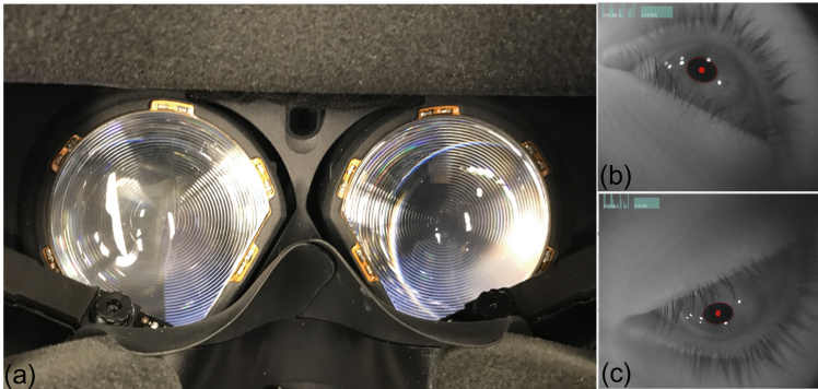
Fig. 4. (a) The Pupils Labs eye tracking. (b–c) It tracks both eyes with a sampling rate of 120 samples second using infrared lights (Color figure online)
