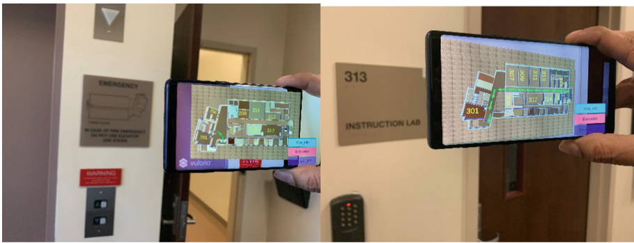
Fig. 5. The 2D evacuation plans and room number signs posted within a building serve as markers to the MARA (Color figure online)
