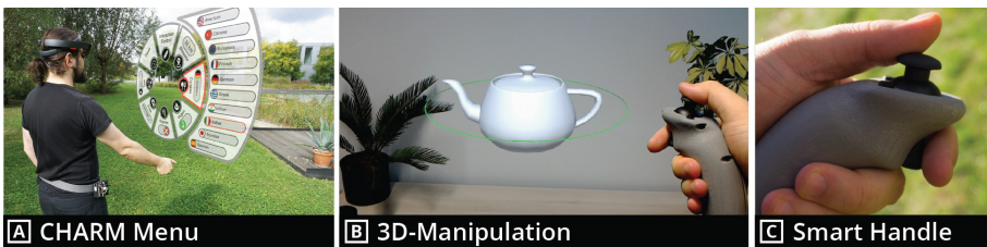
Fig. 1. Our CHARM system is a combination of a versatile retractable input device for radial AR menus (A) and 3D object manipulation (B), that is fully implemented for state-of-the-art AR glasses. The smart handle (C) provides additional controls.
