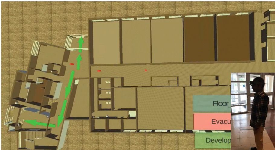
Fig. 1. View of the floor-plan from HoloLens using existing 2D plans and room numbers as markers
