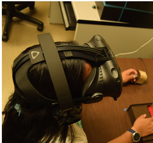
Fig. 3. A mock participant interacting with the experimental user study environment. The participant wears an HTC Vive to view the virtual environment and her left hand is rotating the dial to provide the input for the data collection during the experiment.
